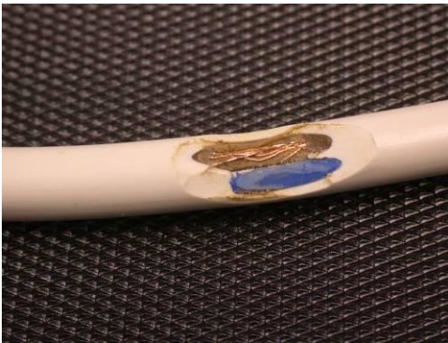
Damage to power cable sheath.
