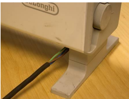
Cable not being gripped.
