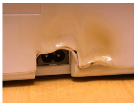
Damage to external casing.
