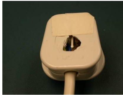
Damage to mains plug.
