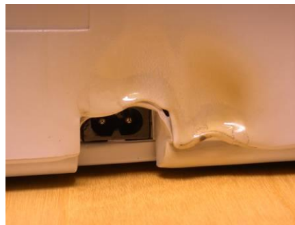
Damage to external casing.
