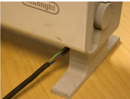
Cable not being gripped.
