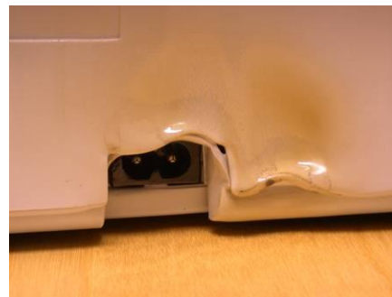
Damage to external casing.
