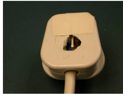
Damage to mains plug.
