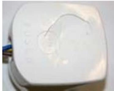
3a Damage to mains plug
