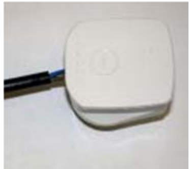
3b Inadequate strain relief
