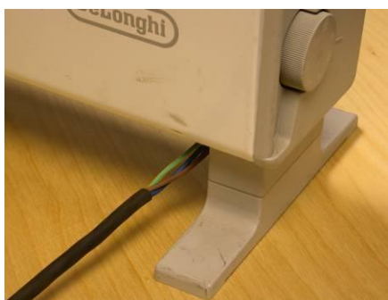
Cable not being gripped.
