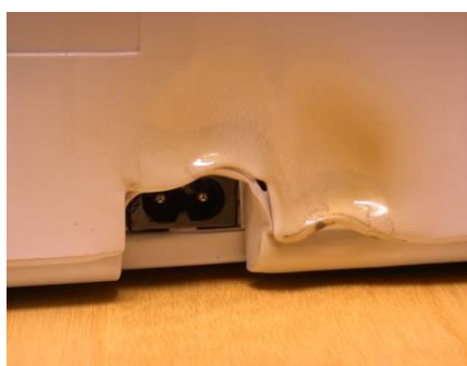
Damage to external casing.
