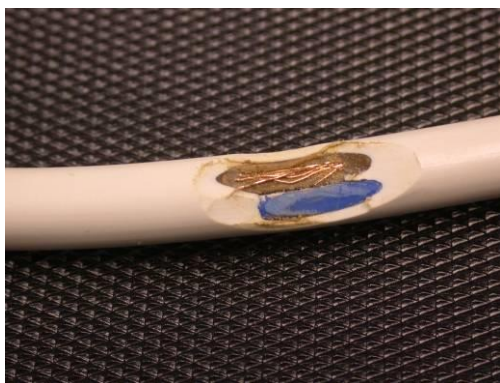
Damage to power cable sheath.
