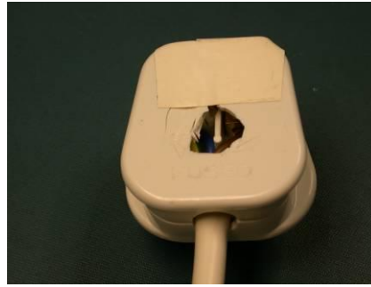
Damage to mains plug.
